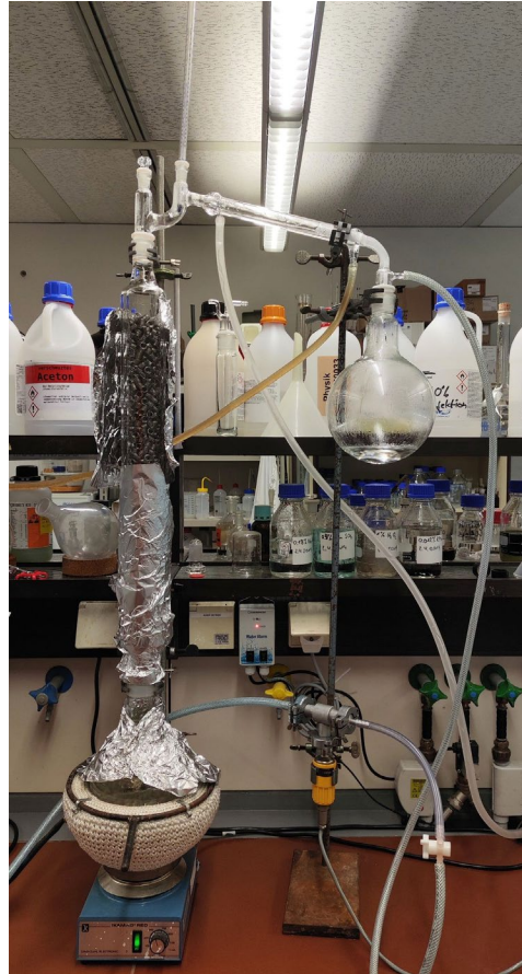
DIN purification using an aluminum oxide column and fractional distillation with Raschig rings
