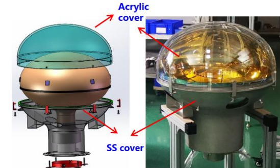
PMT Implosion protection, Acrylic & stainless steel cover (JINST 18 (2023), P02013)
