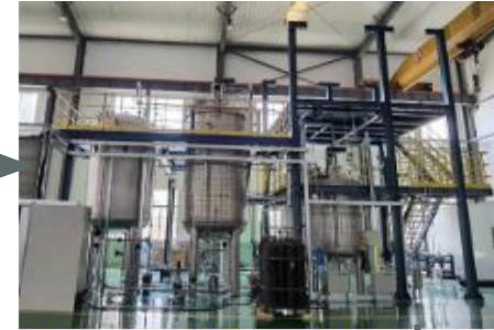
Mixing adds PPO and bis-MSB
