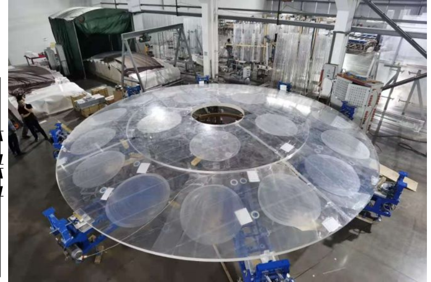
Test fitting of north pole acrylics
